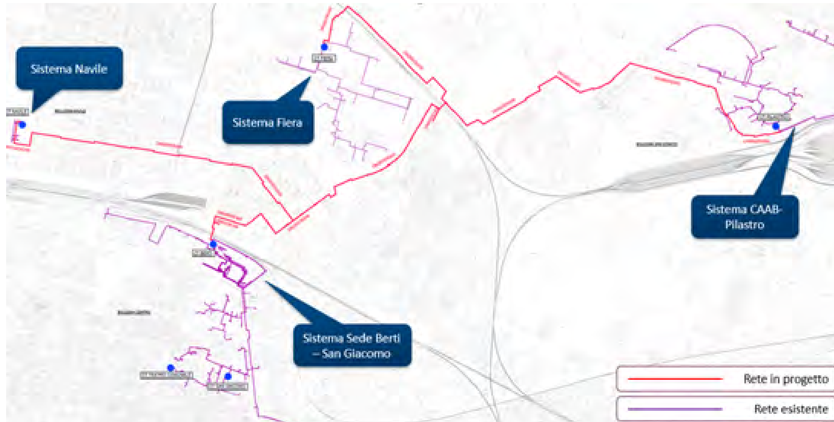
Figure 4.2 – Planned extension of the district heating network of Bologna.
